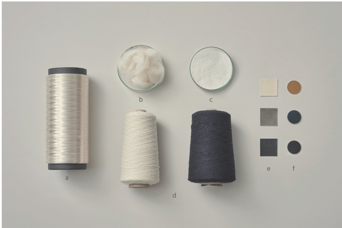
Figure 1-1: Brewed Protein™ materials. Examples of materials that can be formed by processing (c) Brewed Protein polymer, including (a) filament, (b) staple fiber, (d) spun yarn, (e) leather, and (f) resin.
