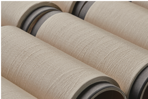
Figure 1-2: Filament yarns produced via dissolving Brewed Protein polymer in a solvent and extruding it through a nozzle. These yarns exhibit a luster and fineness similar to silk.
