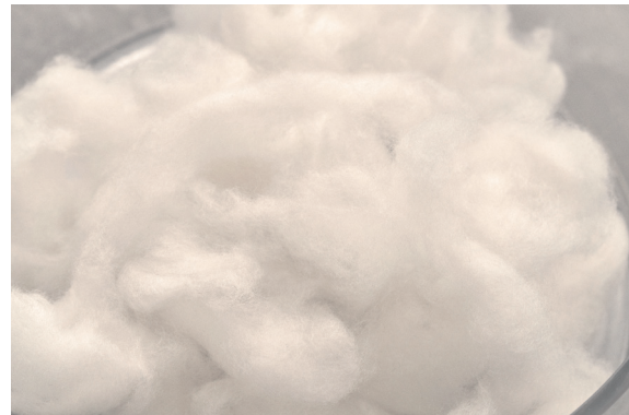
Figure 1-3: Brewed Protein filaments that are cut into short, discrete lengths. The texture of the final material is greatly dependent on the fiber porosity and degree of twisting or entanglement of the staple fibers.
