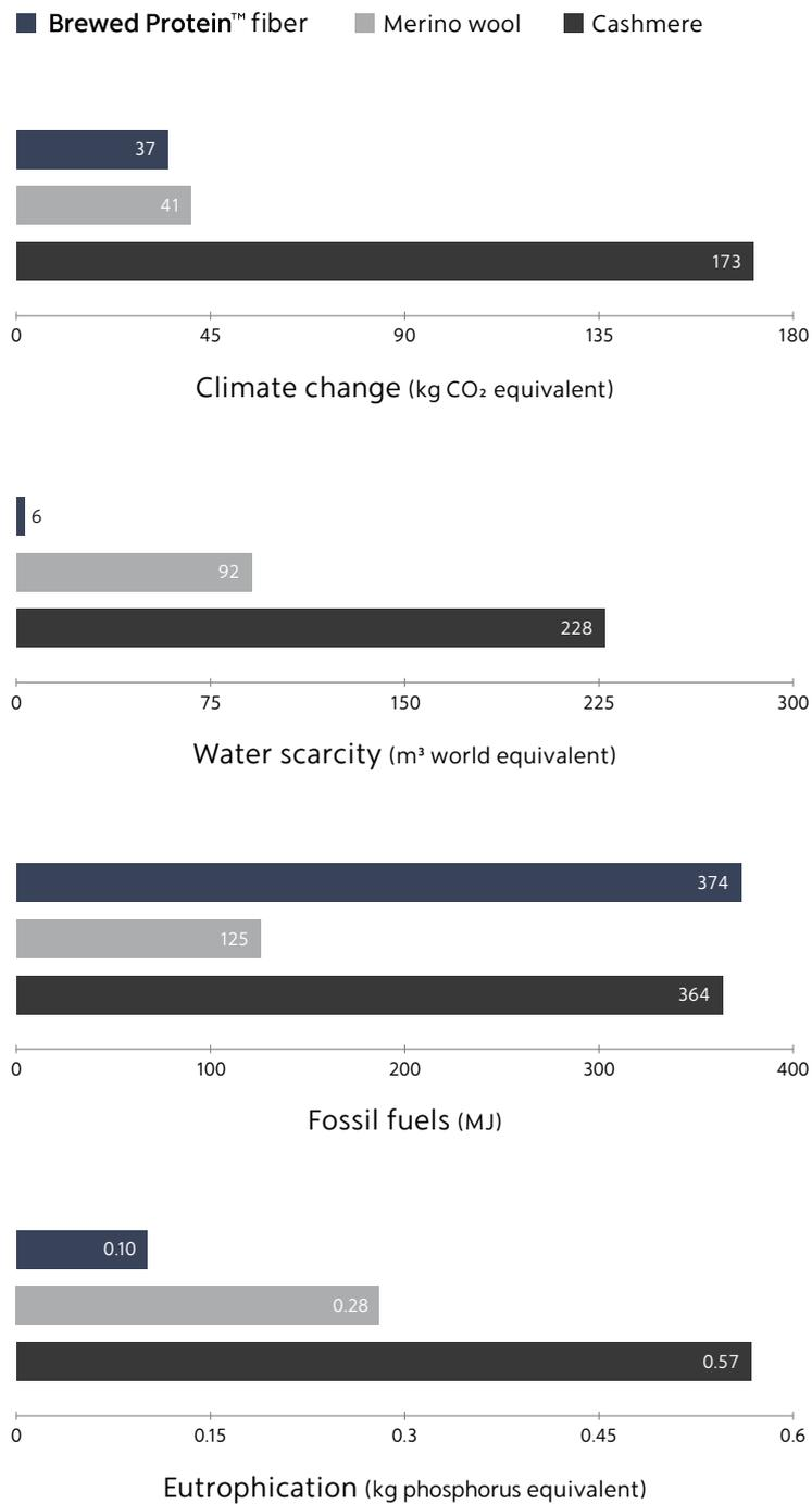
Figure 3: Midpoint results of the cradle-to-gate life cycle impact of producing 1 kg of Brewed Protein, merino wool, and cashmere fiber comparison using the impact indicators used in the Sustainable Apparel Coalition's Higg MSI assessment method.
