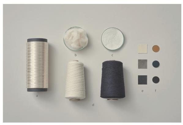
Figure 1-1: Brewed Protein<sup>™</sup> materials. Examples of materials that can be formed by processing (c) Brewed Protein polymer, including (a) filament, (b) staple fiber, (d) spun yarn, (e) leather, and (f) resin.
