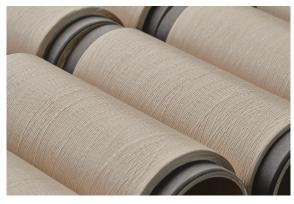
Figure 1-2: Filament yarns produced via dissolving Brewed Protein polymer in a solvent and extruding it through a nozzle. These yarns exhibit a luster and fineness similar to silk.
